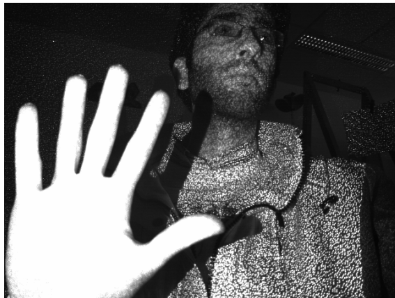
Figure 10: Kinect pattern projection on close objects
