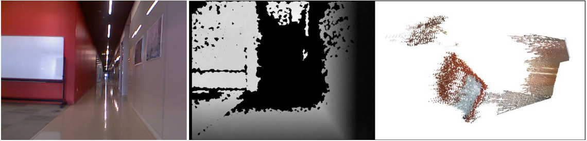
Figure 25: (left-to-right) RGB image, depth image, and the corresponding 3D view. Notice the high level of noise as shown in the 3D image.
