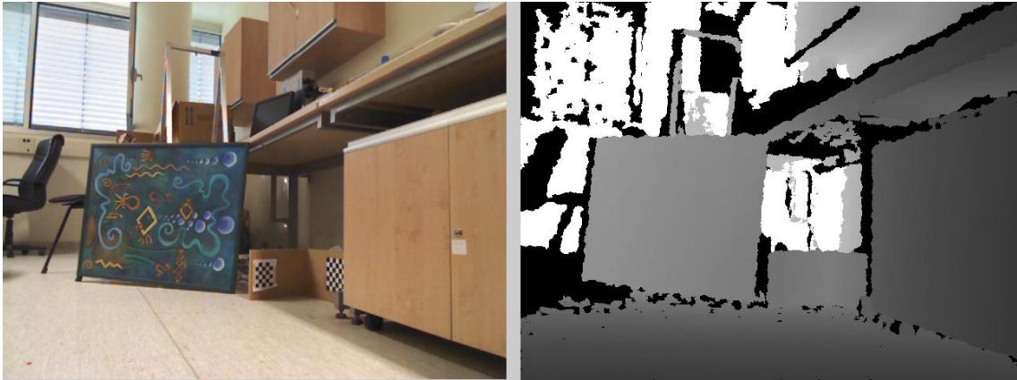
Figure 11: (Left) Color image captured by the Kinect. (Right) Depth image obtained. White and black pixels do not have depth information due to distance or occlusion.
