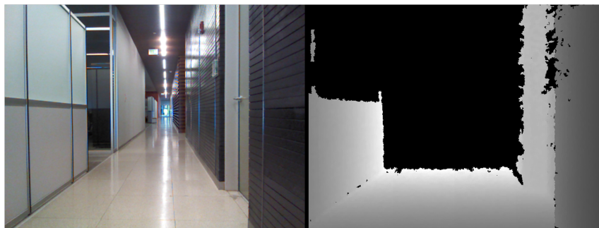
Figure 21: (left) Kinect RGB image. (right) Depth image. Black pixels do not have depth data.
