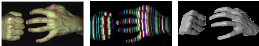
Figure 5: An example of pattern projection for 3D reconstruction using structured lighting
