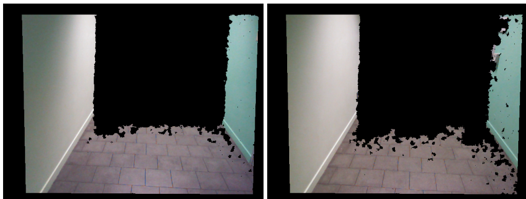
Figure 18: Kinect reliable depth data: Black pixels correspond to areas with unknown depth.
