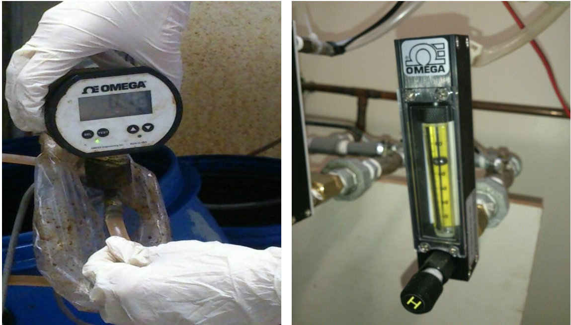
Figure C-7: Pressure sensor (left), rotameter (right)
