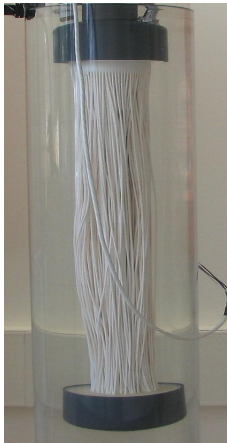
Figure C-6: Flat sheet MBR (left), hollow fiber MBR (right)
