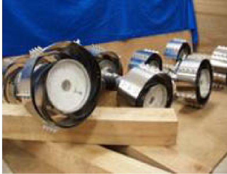
Figure 8: Genbu climbing over a small step using the passive swivel joint
