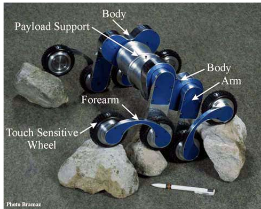
Figure 2: The Octopus Robot with labeled parts
