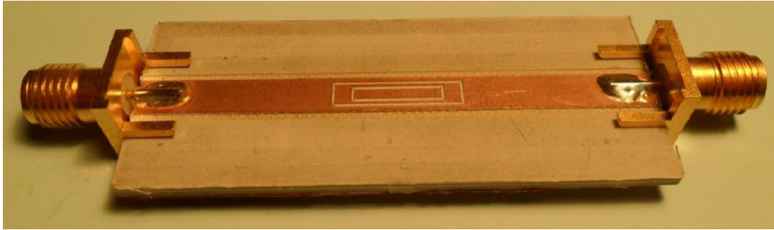
Figure 2.6: Photo of the designed dual stop-band filter
