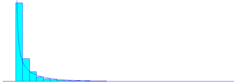
Figure 24: Inter-arrival Time Distribution of walk-in patients to the clinic from Arena Input Analyzer; Beta distribution having a Beta of 0.273, an alpha of 7.48, a multiplier of 484, a distribution mean of 17.04, and distribution standard deviation of 30.15 (minutes)
