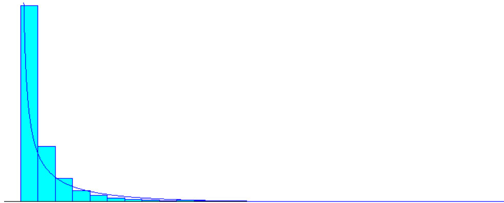
Figure 16: Inter-arrival Time Distribution of walk-in patients to the clinic from Arena Input Analyzer; Beta distribution having a Beta of 0.267, alpha of 7.44, a constant of -0.001 distribution mean of 16.7, and distribution standard deviation of 30 (minutes)
