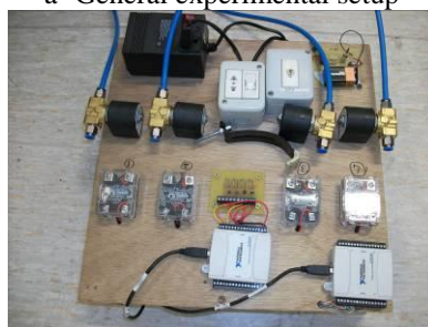
Valve system used for changing out-vehicle sample intake location b- Experimental setup components
