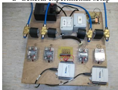
c- Valve system used for changing out-vehicle sample intake location
