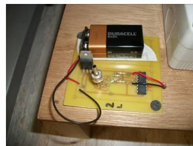
d- Board used for sensing of absolute pressure
