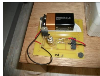
Board used for sensing of absolute pressure
