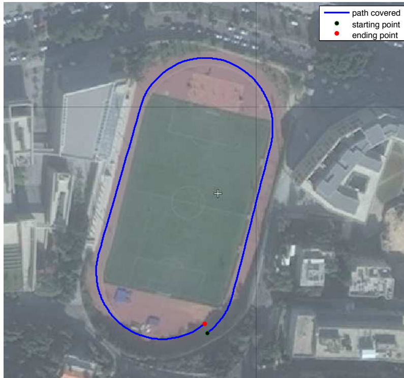
Figure 6.1: Top: picture of the experimental environment (right) and sample texture of the ground (left). Bottom: estimated trajectory using our system for a total run of 461meters.
