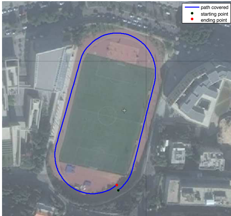
Figure 8.11: Top: picture of the experimental environment (right) and sample texture of the ground (left). Bottom: estimated trajectory using our system for a total run of 418.1 meters. The error is 1.25%
