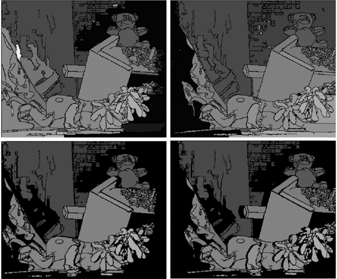
Fig.4.10. Example of Obtained Disparity Maps through SAD Based Segmentation
