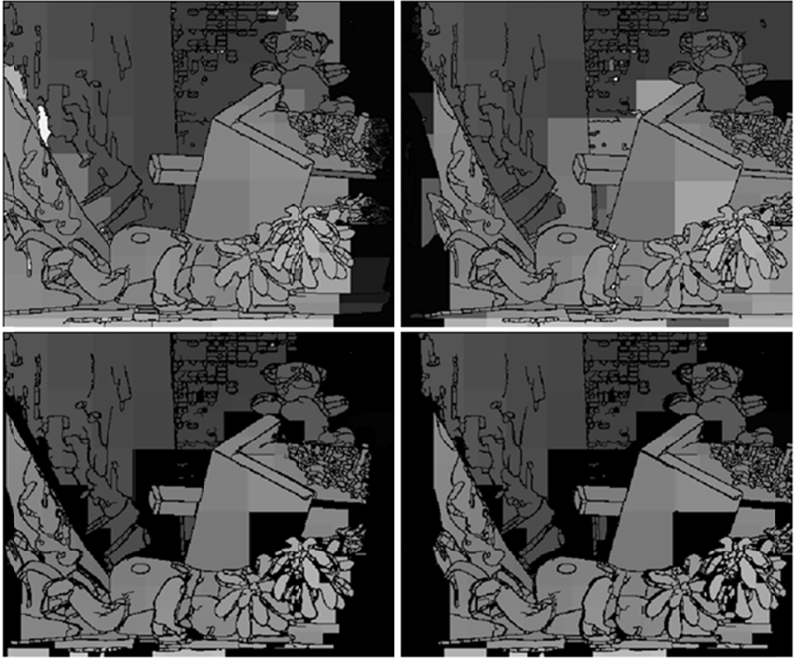
Fig.4.11. Example of Obtained Disparity Maps through SAD Based Segmentation with smaller objects
