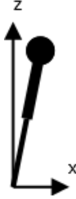
Figure 8: Linear Inverted Pendulum Model with a prismatic joint
