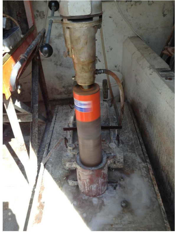
B. 10 Sample being cored
