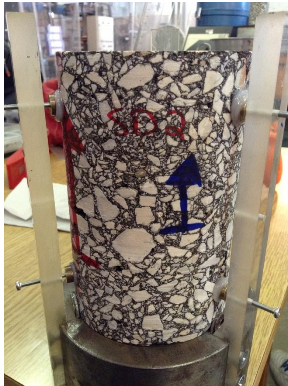
B. 13 Sample being glued
