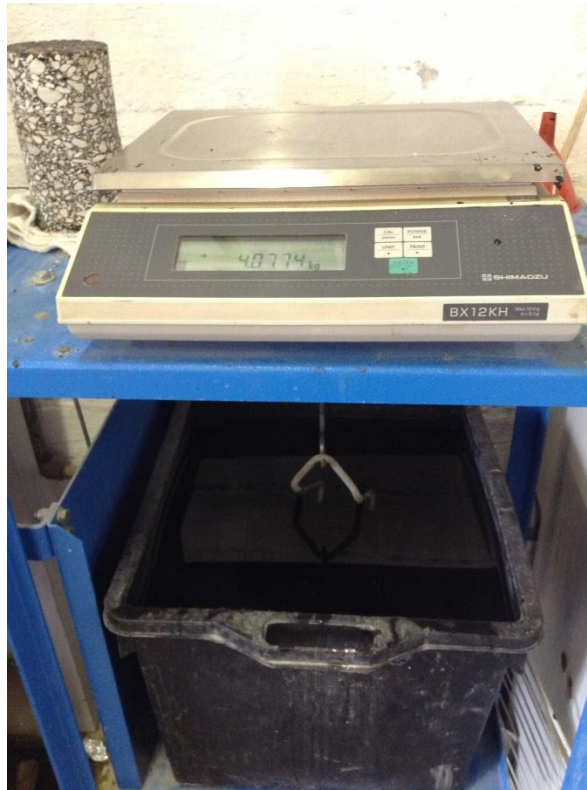
B. 7 Sample submerged in water to measure G_{mb}
