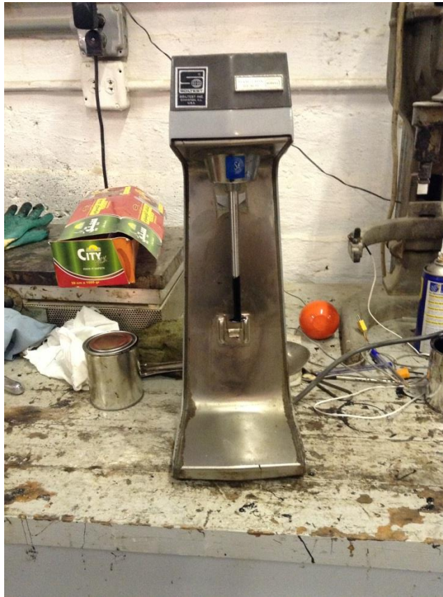
B. 20 Mixer used to prepare the mastic (filler + binder)
