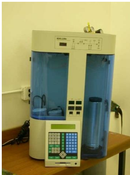
B. 19 BET machine used to measure the surface area of the filler material
