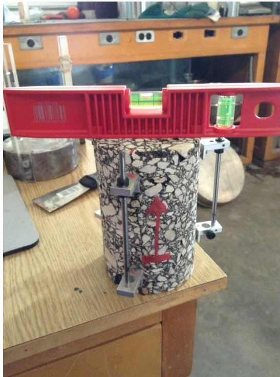
B. 14 Installing brackets
