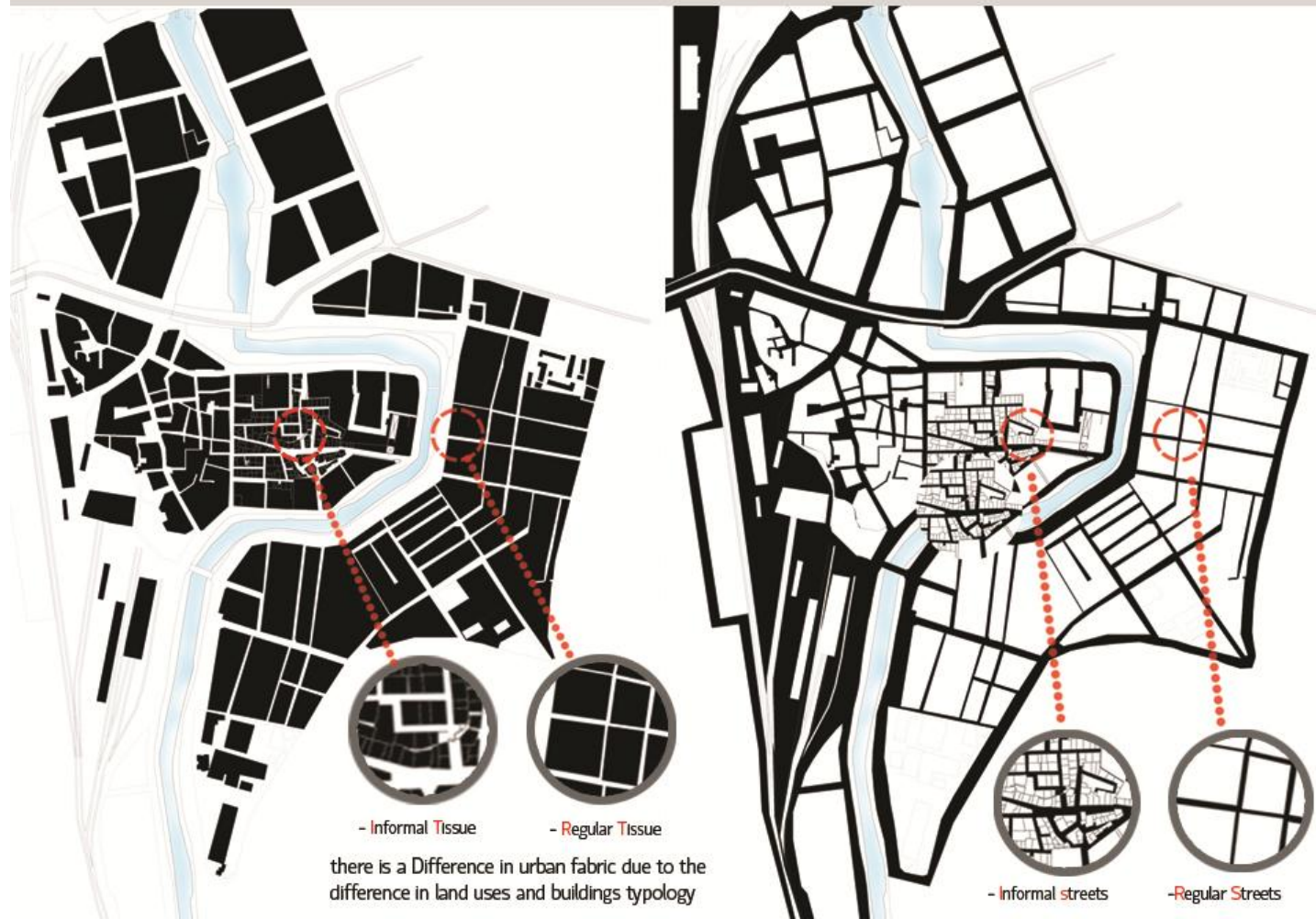
Figure 4.7: Solid/ Void and Nolli maps study the density and different character areas of the site
