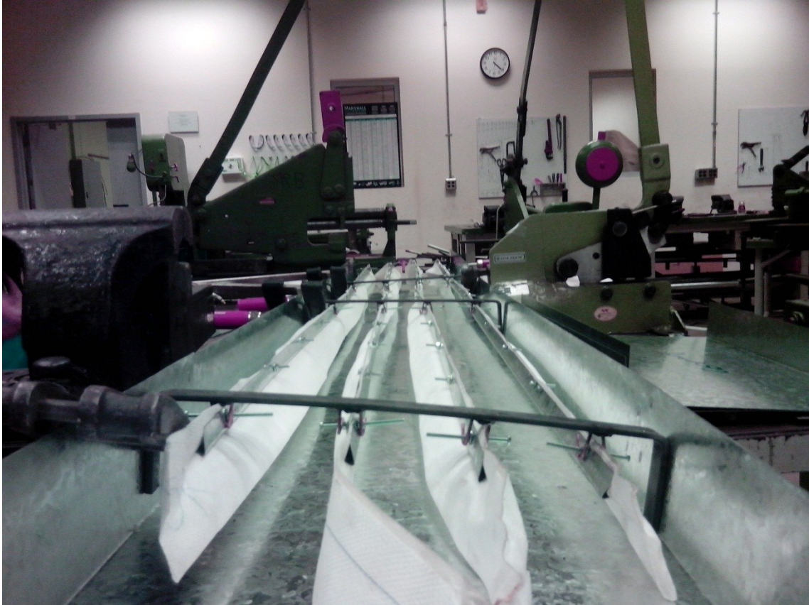
Figure 18: Permeable pipes assembly in the regenerator/dehumidifier
