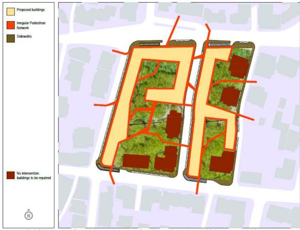
Figure 5.16. Intervention: Plan at Mezzanine Floor Level (1/1000)/ Interlocking urban form (Irregular pedestrian network integrated with the attached buildings). By: H. Awada (2014).
