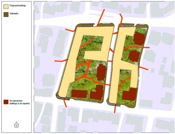
Figure 5.17. Intervention: Plan at typical floor level (1/1000)/ Interlocking urban form (Irregular pedestrian network integrated with the attached buildings). By: H. Awada (2014).
