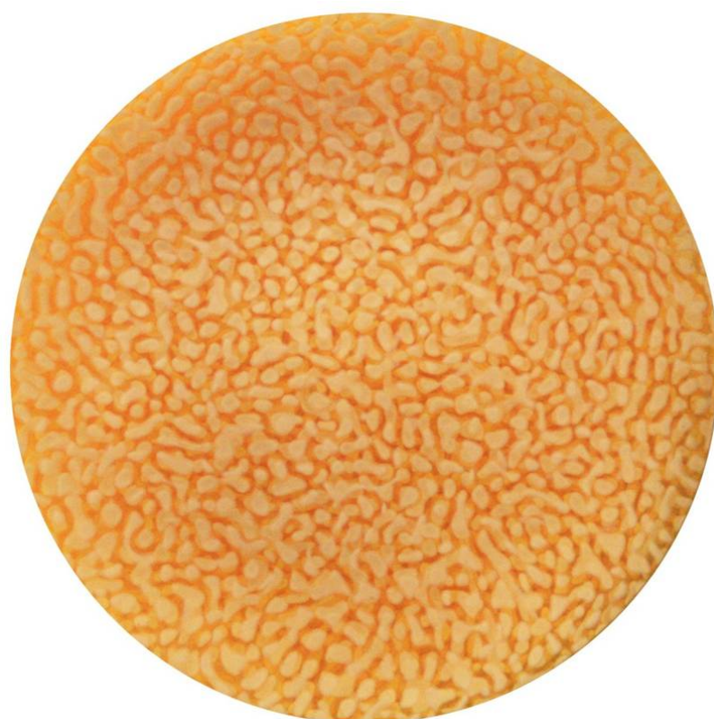
Figure 46: Stationary island-like pattern obtained at 60 mM [\text{Cd}^{2+}]_0 and 200 mM [\text{S}^{2-}]_0 . Gelatin = 5%; Temp = 22 °C.
