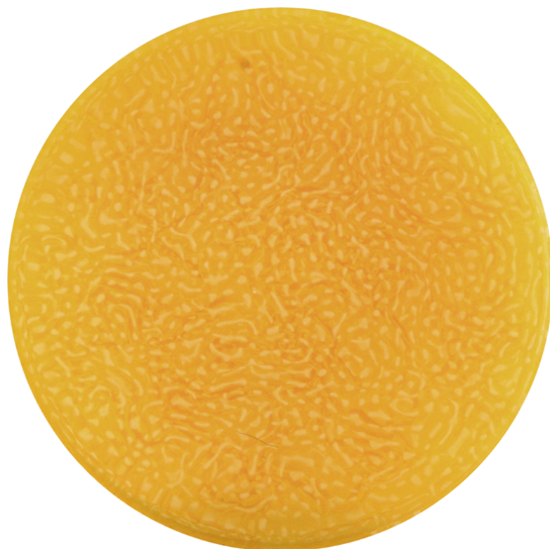
Figure 47: Mixed state of stripes and spots obtained at 60 mM [\text{Cd}^{2+}]_0 and 350 mM [\text{S}^{2-}]_0 . Gelatin = 5%; Temp = 22 °C.
