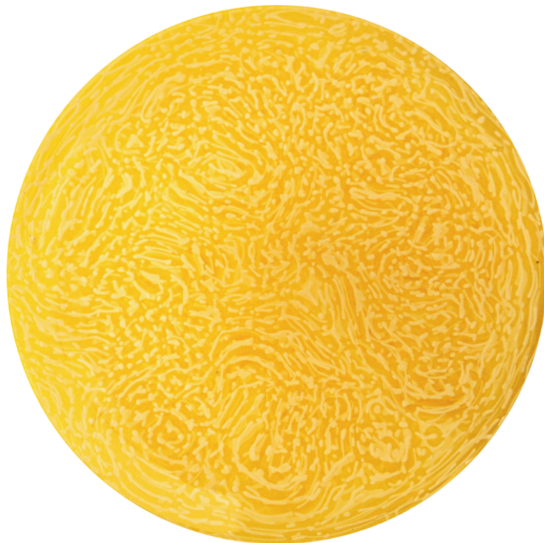
Figure 45: Labyrinthine pattern obtained at 40 mM [\text{Cd}^{2+}]_0 and 200 mM [\text{S}^{2-}]_0 . Gelatin = 5%; Temp = 22 °C.
