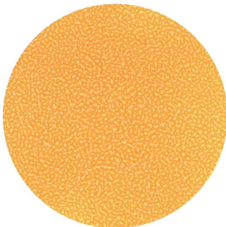
Figure 48: Spot-like pattern obtained at 80 mM [\text{Cd}^{2+}]_0 and 300 mM [\text{S}^{2-}]_0 . Gelatin = 5%; Temp = 22 °C.
