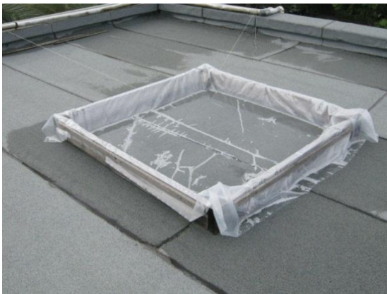
Figure 7. 2.1 \text{m}^2 tarpaulin for muddy rain collection.
