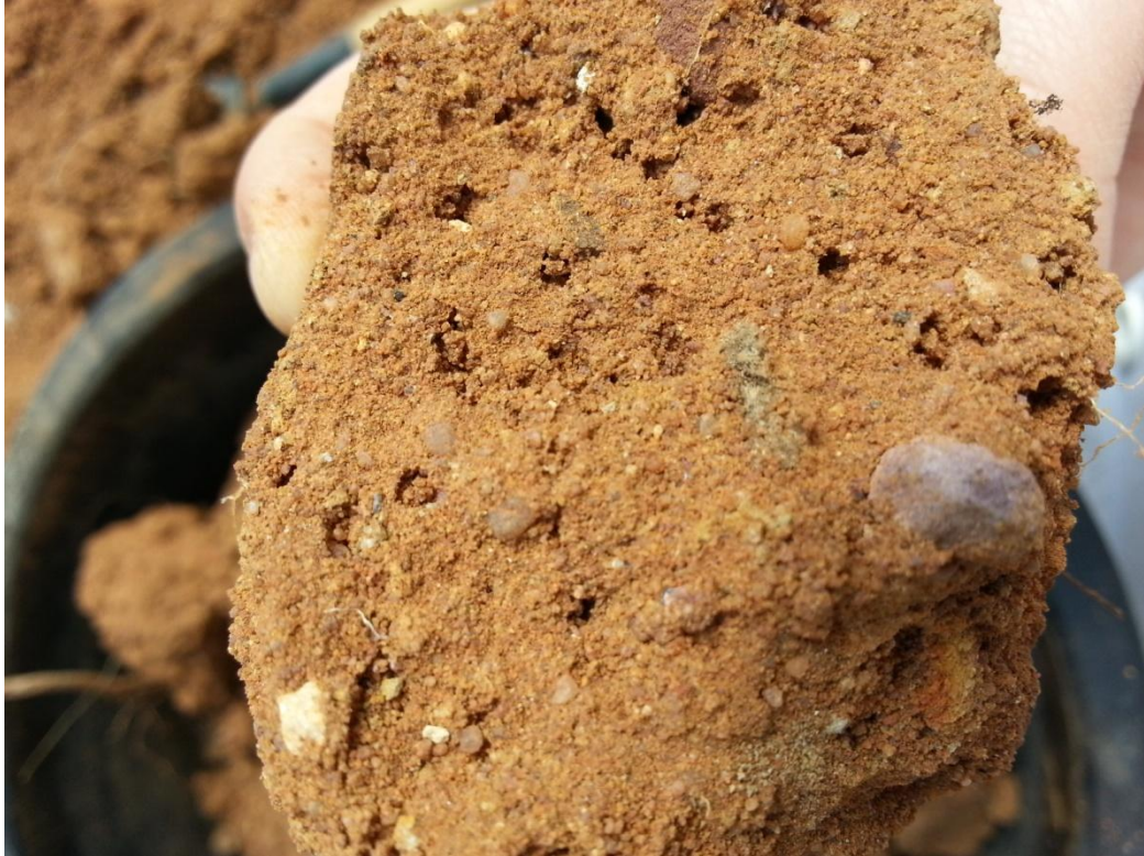
Figure 11: Pores left by shrunken hydrogel particles in Sandy Clay soils 21 weeks after planting.
