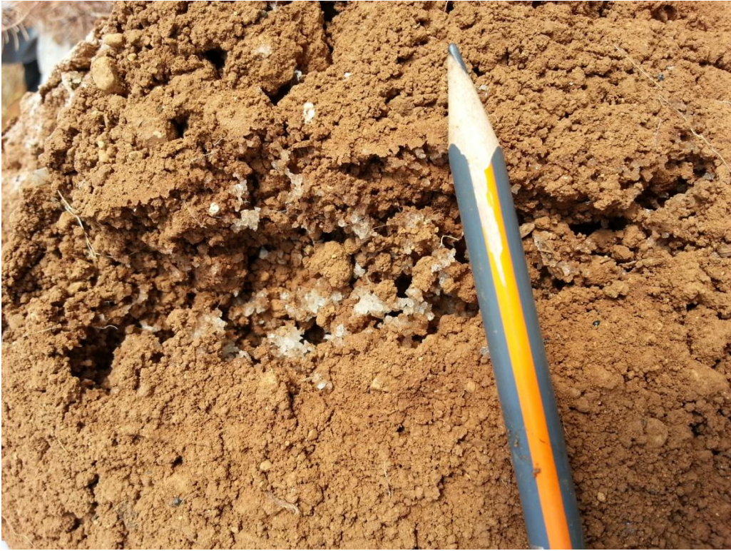
Figure 10: The air pocket formed by the layer of hydrogel in clay soils 21 weeks after planting
