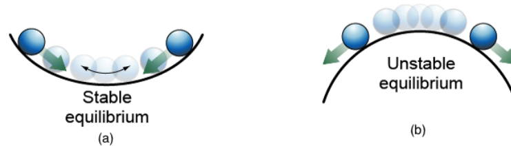
Figure 16: (a) A perturbation to the system in a stable equilibrium results in the return to the stable position. (b) A perturbation in the unstable equilibrium results in the escape away from stable position.
