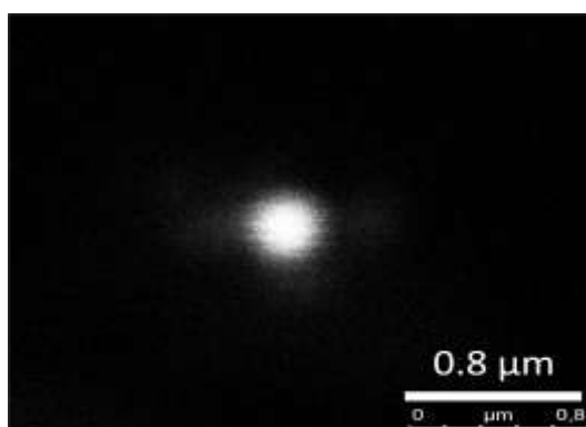
Figure 2.7. STED confocal fluorescence image of the nanocapsule. The excitation wavelength was 430 nm and the emission wavelength was 430 nm and the emission was collected using a band filter in the range of 460-600 nm.
