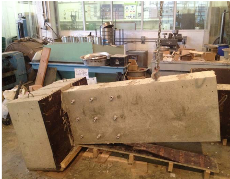
Figure 8. Formwork removed and specimen is erected
