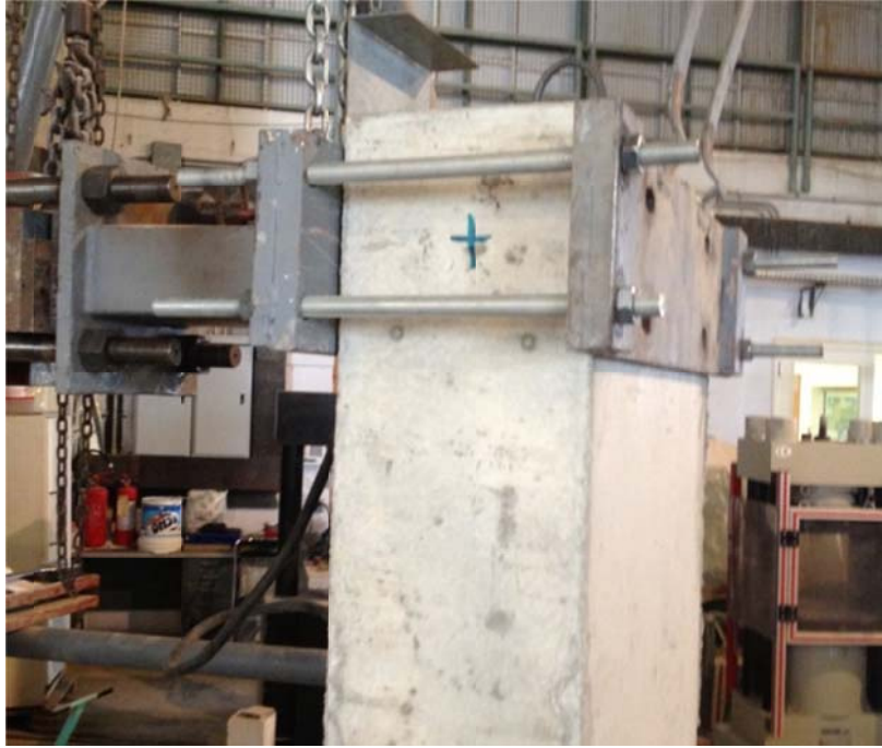
Figure 4. Lateral load applied at an effective height of 150 cm of the specimen.
