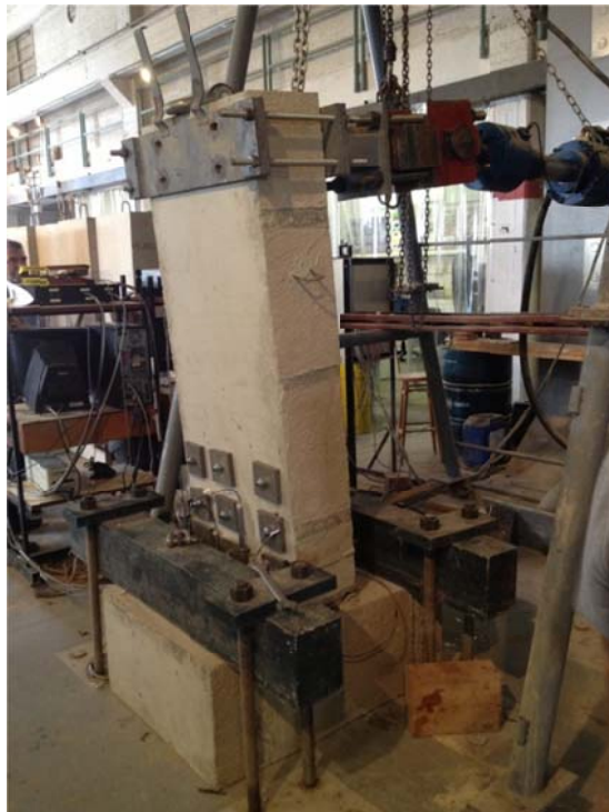
Figure 12. Maximum push cycle causing specimen W20-SA to tilt.
