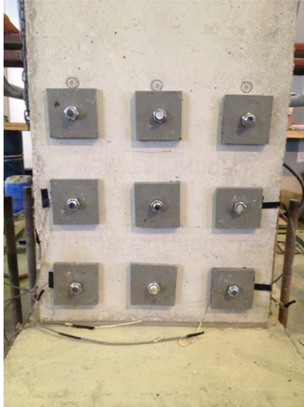
Figure 14. Steel plates configuration and wiring connections of the strain gauges for specimen W20-SA
