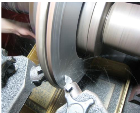
Fig. 3. Brake disc skimming and iron boring scrap collection.
