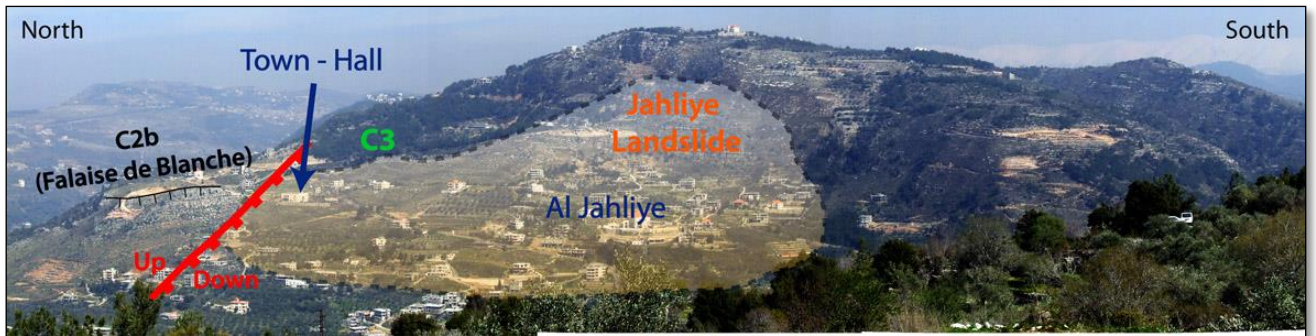
Figure 3.18: Panoramic View of al Jahliye, showing the Jahliye-Ain el Haour Fault as it juxtaposes the C3 and C2b. This fault passes on the northern boundary of the Jahliye Landslide. (See location 3 of Fig. 3.16).
