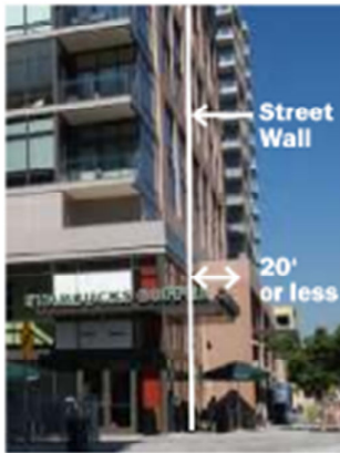
Walls above the ground floor that step back less than 20' from the ground floor street wall are part of the street wall, as illustrated above.
