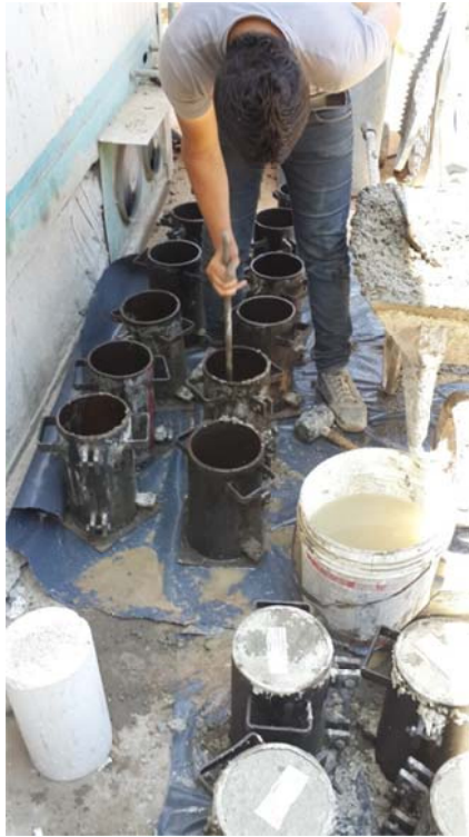
Figure 8-11: Preparing cylinders for testing the compressive strength
