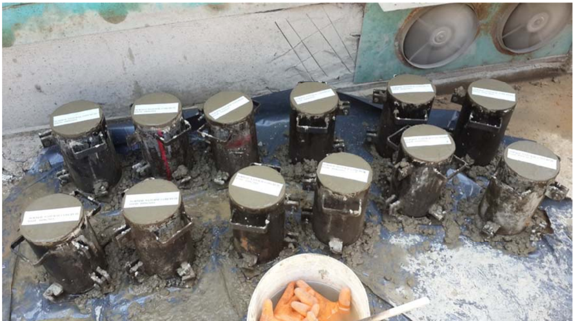
Figure 8-11: Preparing cylinders for testing the compressive strength
