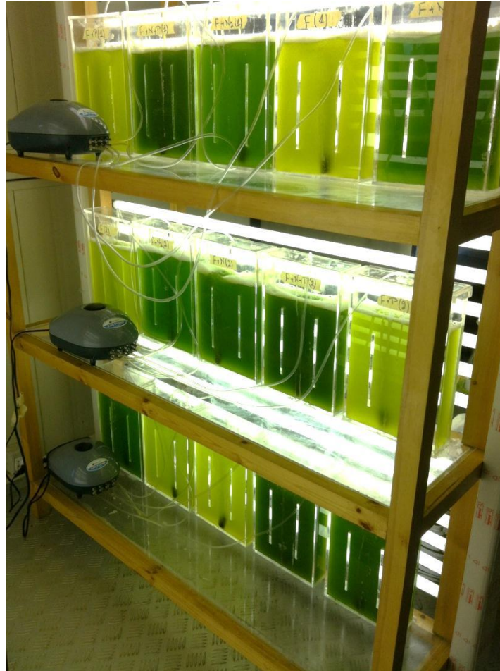
Figure 57. Flat bioreactors used to study the effect of N and P on the growth of Amshit isolate experiment.
