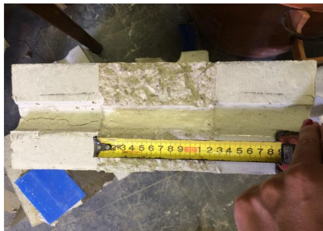
Figure 14. Pullout failure of fully confined specimens
