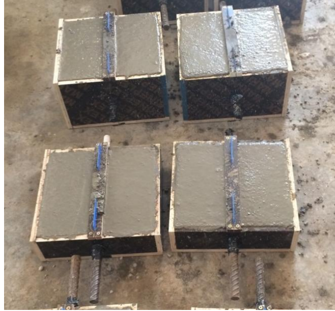
Figure 6. Test specimens after casting
