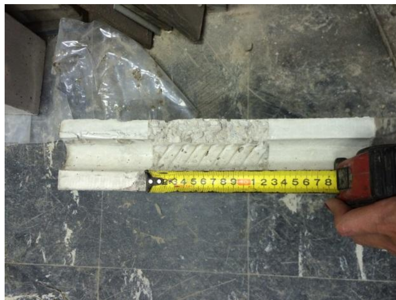
Figure 13. Splitting failure of the unconfined control specimens
