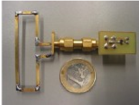
Figure 6. RF harvesting device with a folded dipole reception antenna [10]
