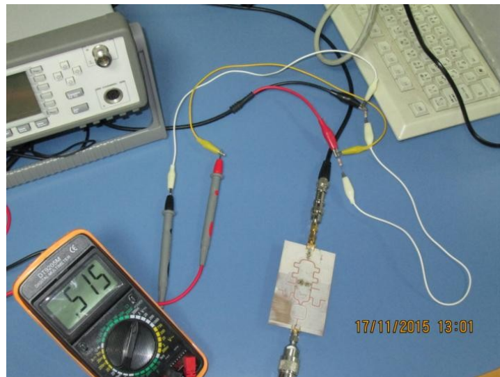
Figure 90. Measured output DC of 515\text{mV} at 0\text{dBm} input power for a 600\Omega load
