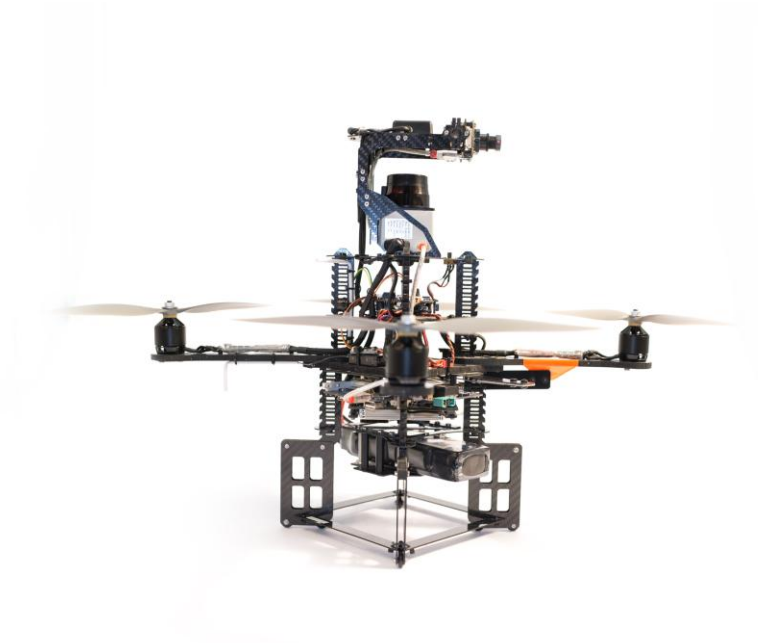
Figure 1: A quadrotor showing the chassis and the four rotors and propellers
