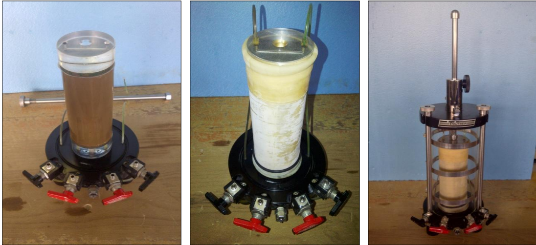
Figure 3.12: Preparation of Achrafieh clay specimen for triaxial testing
