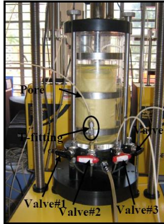
Figure 4.14: Flushing of the drains
