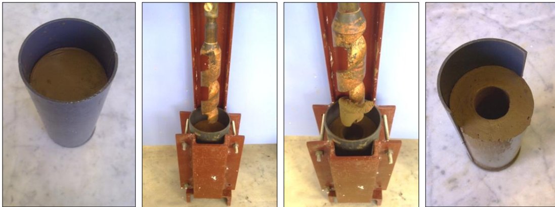
Figure 3.13: Augering apparatus of Achrafieh clay specimens
