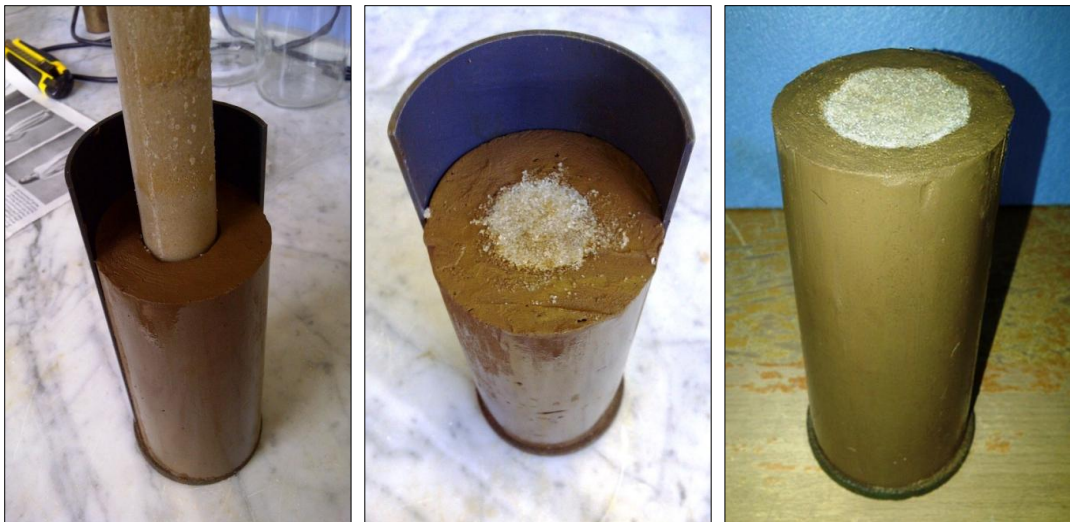
Figure 3.15: Photographs presenting the process of preparing and installing sand columns
