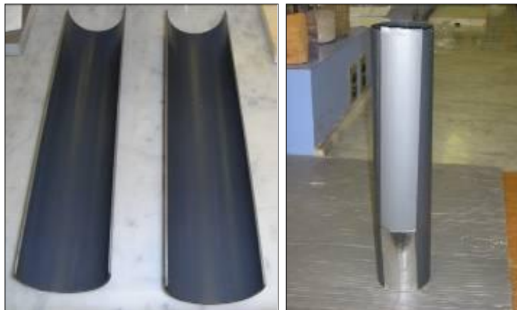
Figure 3.9: Split PVC pipe and wrapped PVC pipe with duct tape
