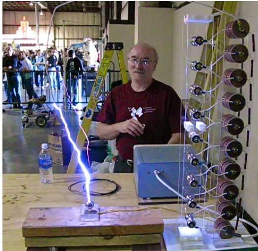
Figure 2.13: Marx generator in action, 600K volts derived from 6 C cell batteries [30]
