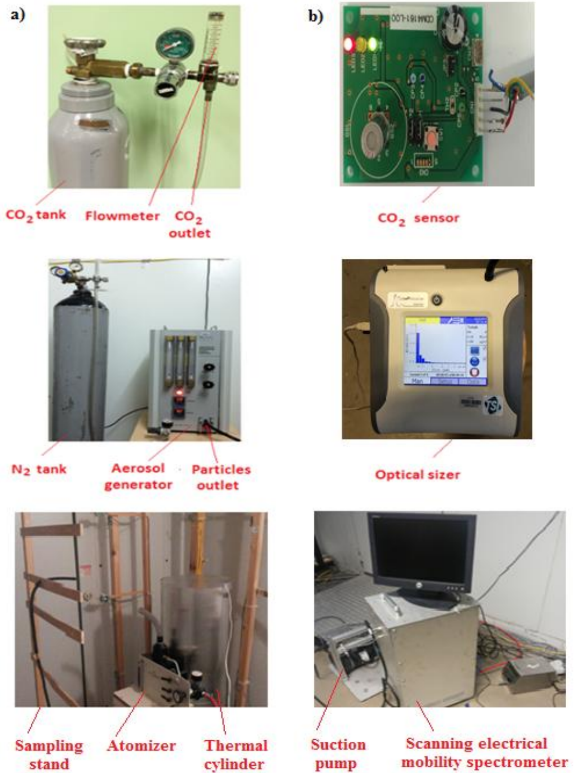
Fig. 4.2: Equipment of CO 2 and particles: a) generation; and b) concentration measurement.
