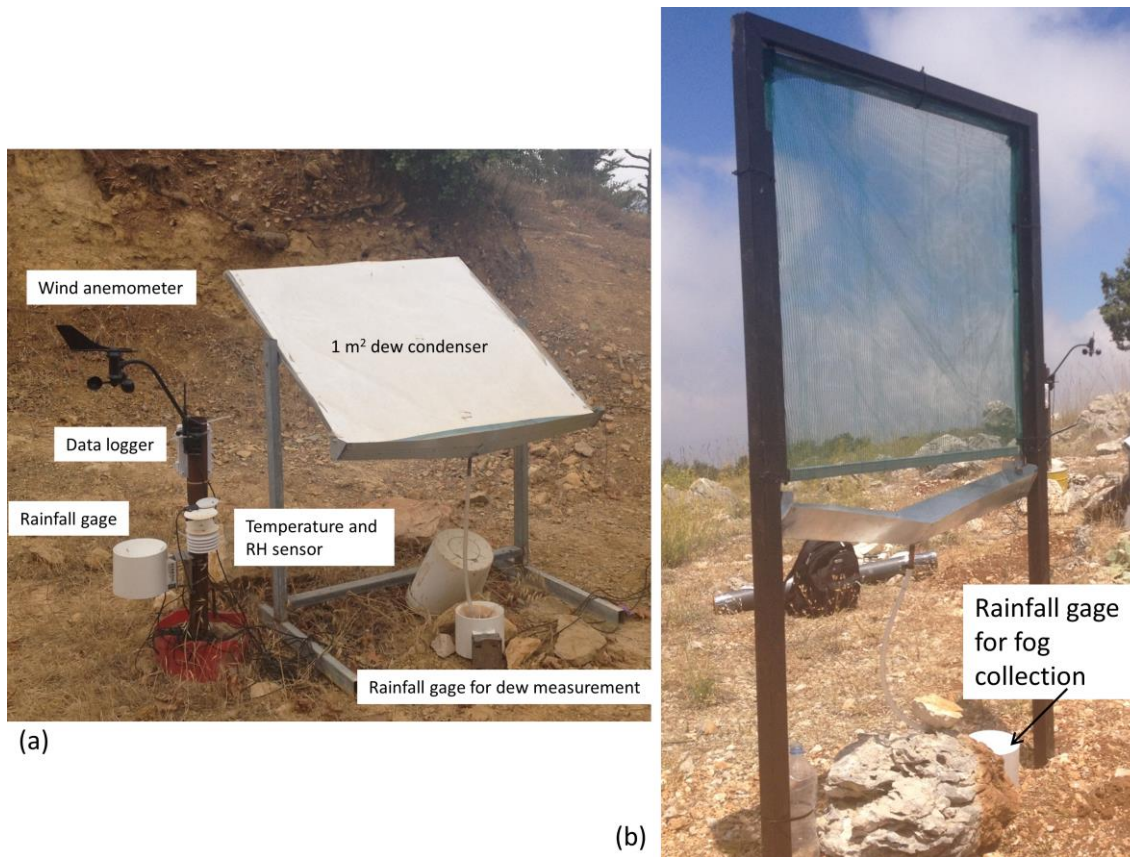
Figure 3.2. (a) Typical dew harvesting station; and (b) Fog harvesting station
