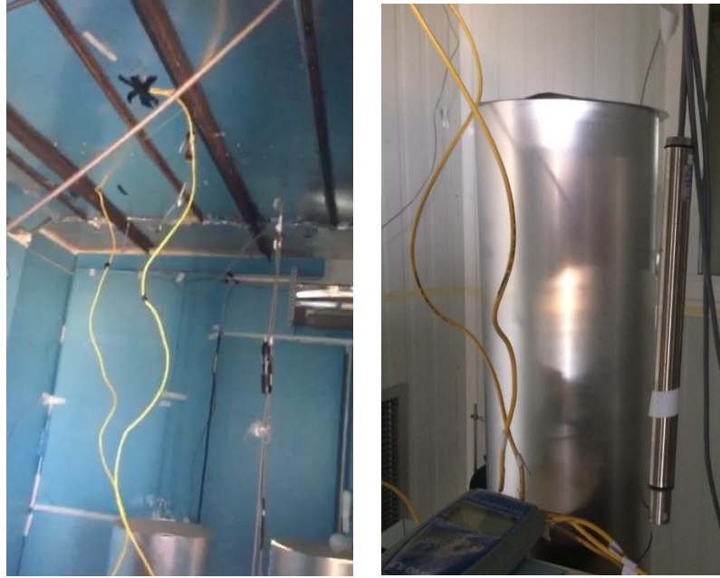
Figure 5: (a) Ceiling and Chamber of the Experimental Setup; (b) A Metallic Cylinder and Data Logger
