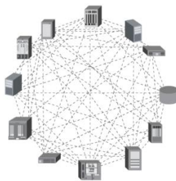
Figure 4. Connection Mesh established by the Diameter Protocol
