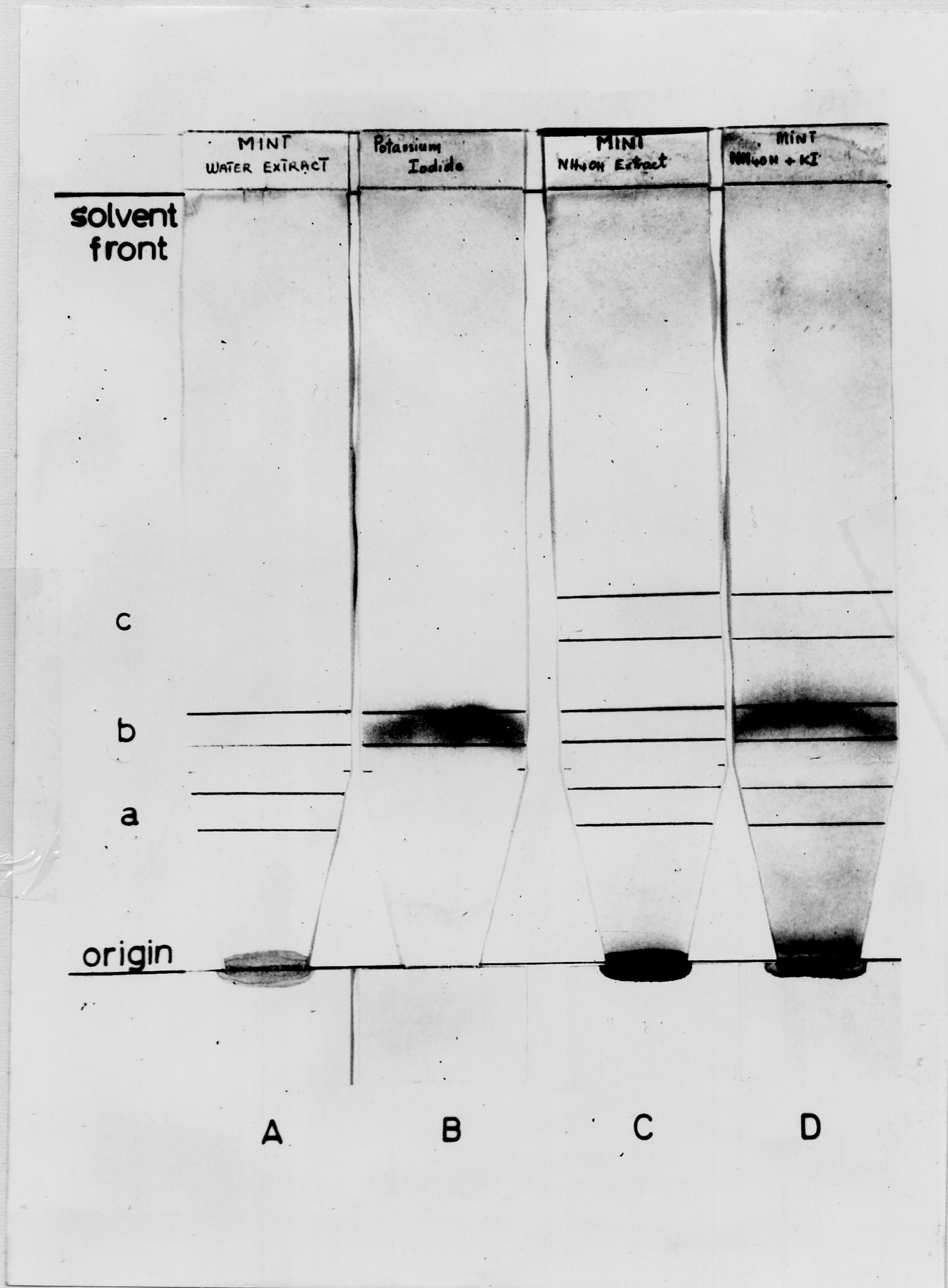
Figure 1. FFCA peaks on paper chromatograms of mint plant extracts chromatographed in n-butanol/acetic acid/water solvent system.
