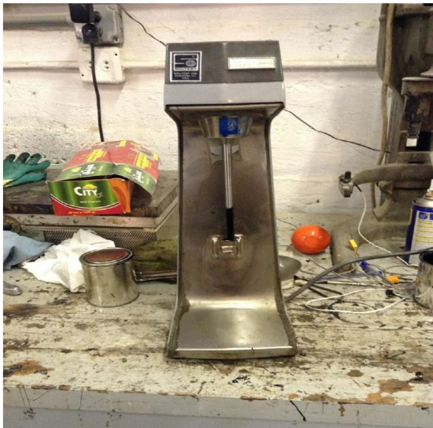
B 6 Mixer Used to Prepare the Mastic (Filler + Binder)
