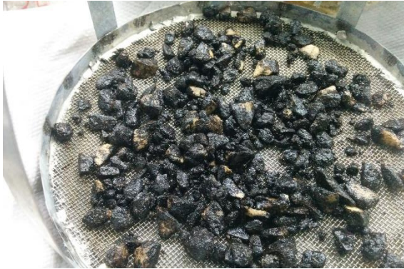
Figure 8 Conditioned sample after the UAMC testing.
