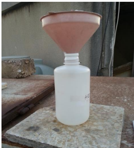
Setup used to collect rainwater for physicochemical testing
