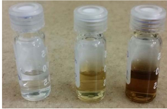
Figure 22: Diclofenac solution color change after exposure to sunlight
