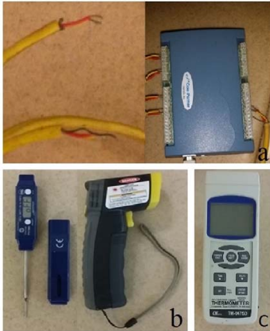
Figure 8 a: Type-K thermocouple and data acquisition unit b: Hand-held thermometers c: Data logging thermometer
