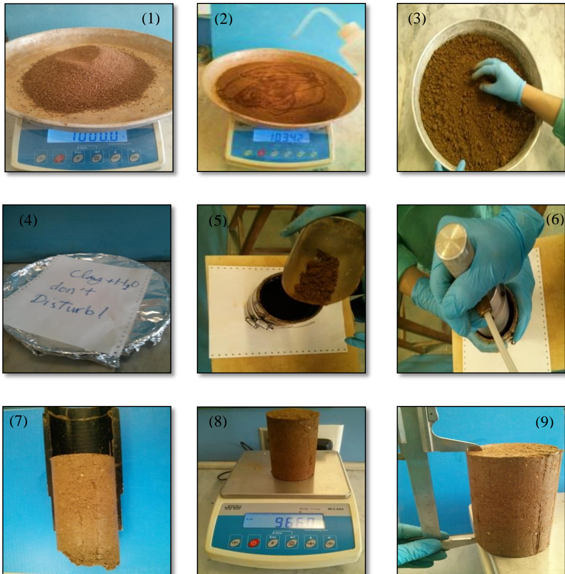
Figure 3.5 Procedures of compacted clay sample preparation.
