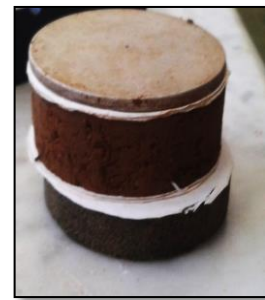
Figure 3.7 Step by step procedure to trim a sample from the compacted clay .
