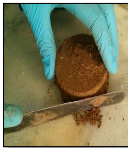
Figure 3.7 Step by step procedure to trim a sample from the compacted clay .
