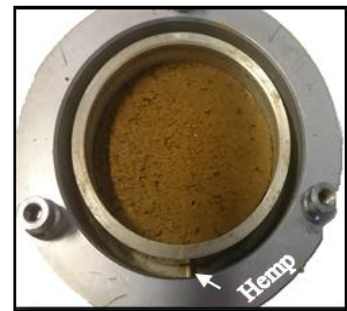
Figure 3.22 Step by step procedure for preparing the sample in the pullout mold.
