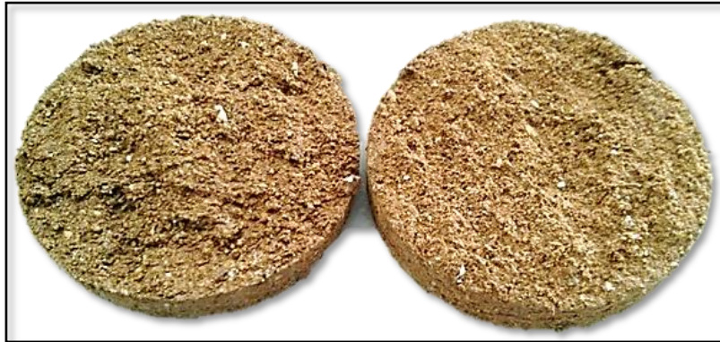
Figure 3.16 Horizontal failure plane of a sheared sample.
