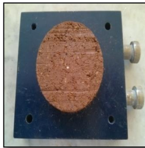
Figure 3.7 Step by step procedure to trim a sample from the compacted clay .
