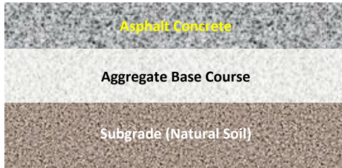
Figure 2.1: Typical three-layered pavement cross-section.
