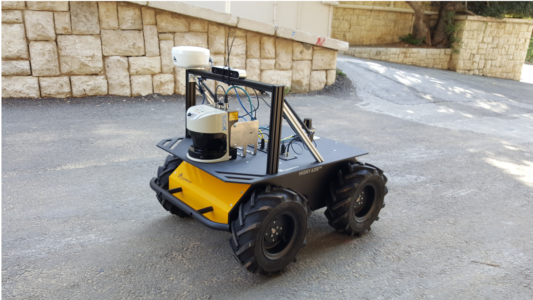
Figure 5.1: Deployed sensors and robot. The Zed Stereo Camera is rigidly mounted on top of the Clearpath Husky UGV.
