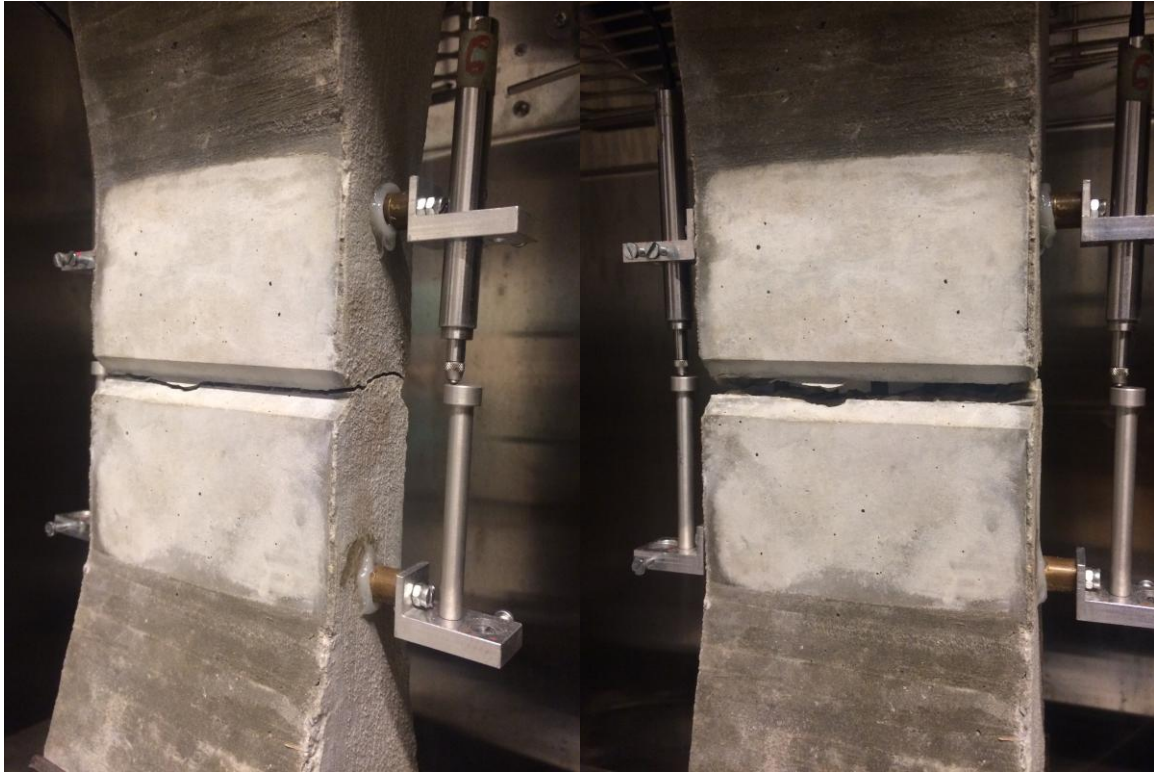
Figure 3-12 Geogrid reinforced concrete mode of failure
