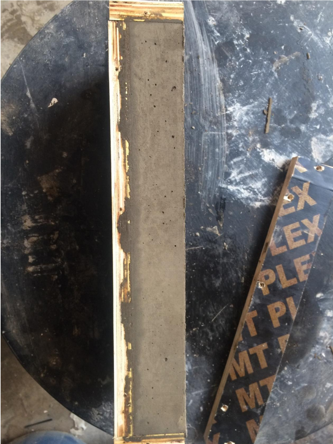
B.2 No separation or major surface voids were observed after de-molding
