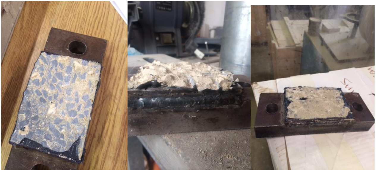
A.2 Typical localized failure at the concrete/epoxy interface
