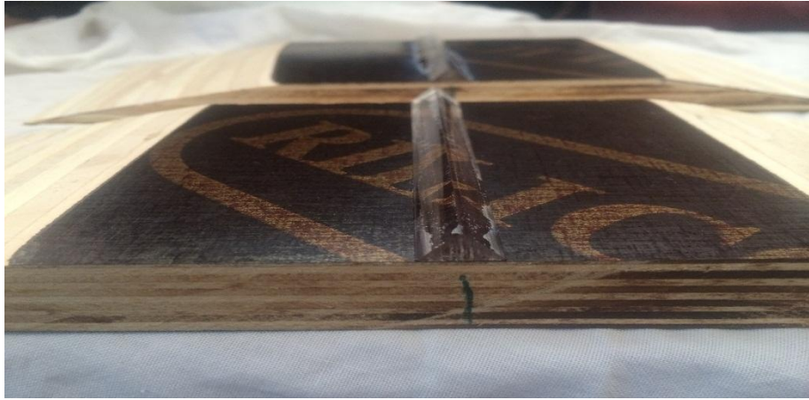
A.13 Gluing the notch
