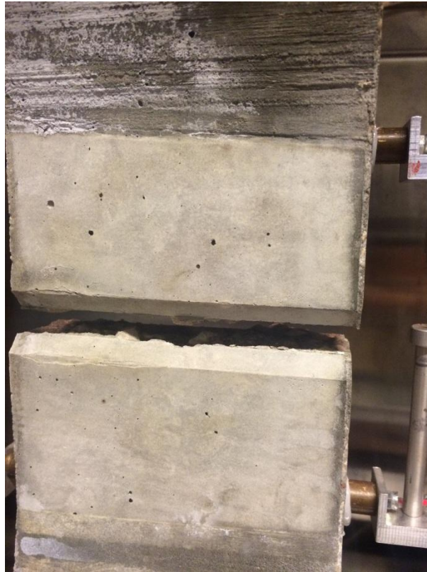
Figure 3-11 Plain concrete mode of failure
