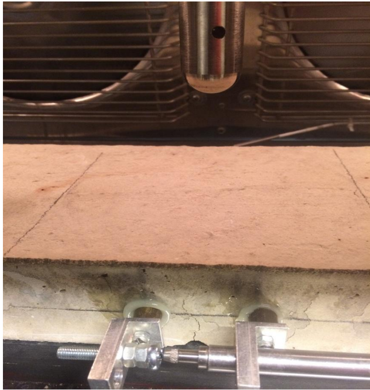
B.10 Geogrid reinforced sample (G-m-1)
