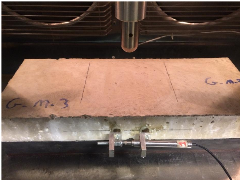
B.12 Geogrid reinforced sample (G-m-3)
