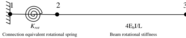
Figure. 12. Equivalent rotational system
