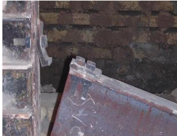
Figure. 3. Von Mises stress contours vs. experimental results: (a) Tension bolt failure (Exp.1 and Exp.1-w), (b) Top angle failure (Exp.2 and Exp.2-w).
