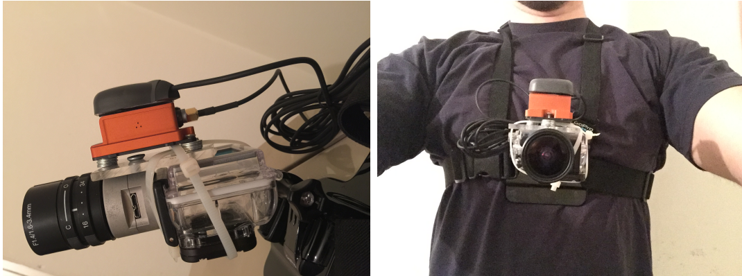
(a) the GPS antenna is fixed to the back of the Xsens INS which is bolted on a small chassis on top of the basler camera.
