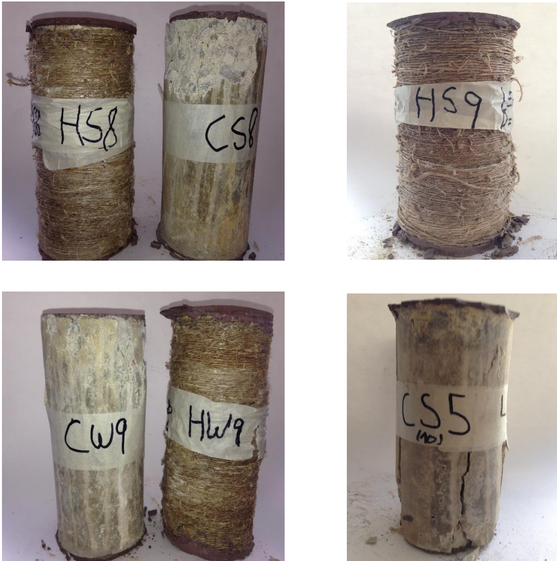
Figure 20: Failure modes of unwrapped and wrapped cylinders
