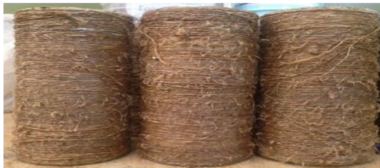
Figure 5: Hemp-fiber confined concrete
