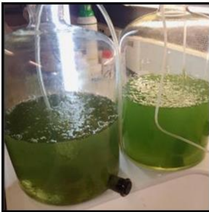
Figure A3. Culturing setup adopted for the cyanobacteria inhibition experiments
