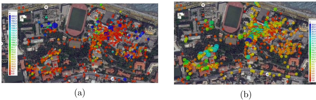
Figure 5.17: Aggregate number of (a) contacts [legend: red - green \rightarrow \leq 50 ; blue \rightarrow \geq 125 ](b) connected pairs [legend: red - green \rightarrow \leq 10 ; blue \rightarrow \geq 17 ] on AUB campus during summer
