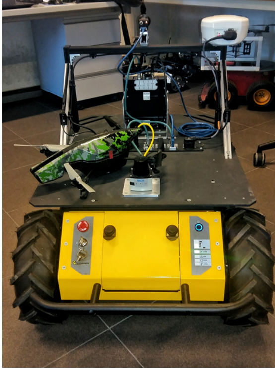
Figure 1.1: The Clearpath Husky robot in our vision and robotics lab equipped with a monocular camera is used during experimentation. The 2D lasers on the robot were not used in the experiment.
