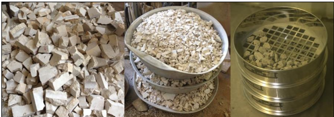
Figure 4.3: Crushing of limestone cores and sieving of limestone aggregates.
