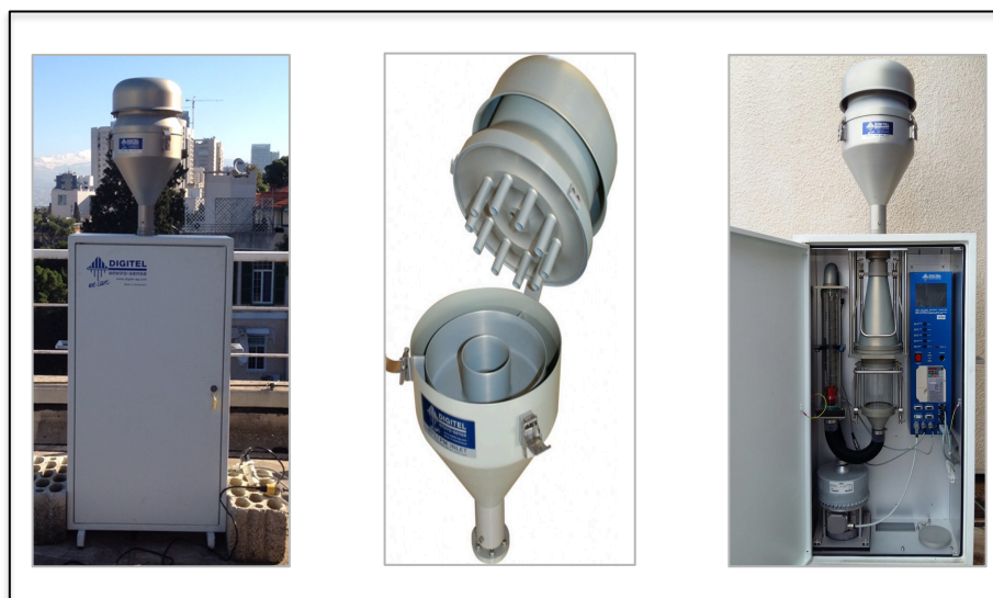
Figure 2.1: from left to right: the high volume sampler, the sampling probe, and the filter and PUF compartments constituting it
