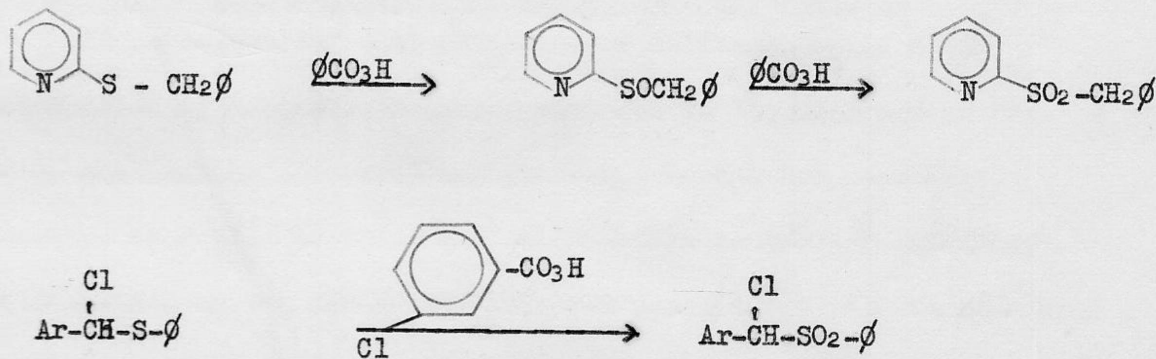
Organic hydroperoxides usually oxidize organic sulfides to the sulfoxide stage only. Recently, however, Kuhnlen obtained high yields of sulfones by the use of metal oxides as catalysts.<sup>33</sup>
