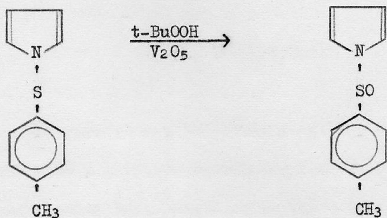
The structure assigned to the product of this reaction is supported by its elemental analysis, its infrared spectrum which contains an absorption band at 1040 cm<sup>-1</sup> (-S- group)<sup>35</sup>, and its further oxidation to 1-(p-toluenesulfonylpyrrole) with hydrogen peroxide in the presence of acetic acid and sodium acetate.
