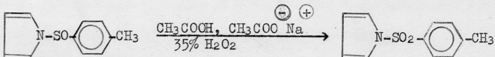
To 0.34 g of 1-(p-toluenesulfinyl) pyrrole was added 0.49 g of sodium acetate, 2 ml of glacial acetic acid and 4 ml of 35% hydrogen peroxide. After the mixture had been stirred for 24 hours with a magnetic stirrer, it was diluted with 20 ml of water and filtered to yield 0.22 g (60%) of 1-(p-toluenesulfonyl) pyrrole, m.p. 100 - 101°.
